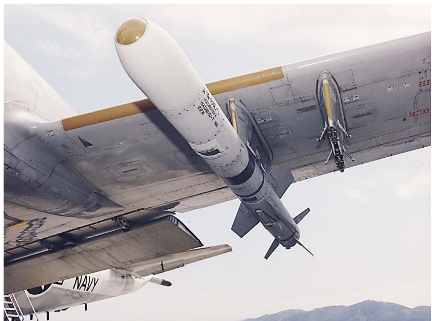
Figure 13. AGM-84E stand-off land attack missile (SLAM) on a P-3C (photograph courtesy of CAPT K. Hohl, Chief of Staff, Commander, Patrol Reconnaissance Force Pacific).
