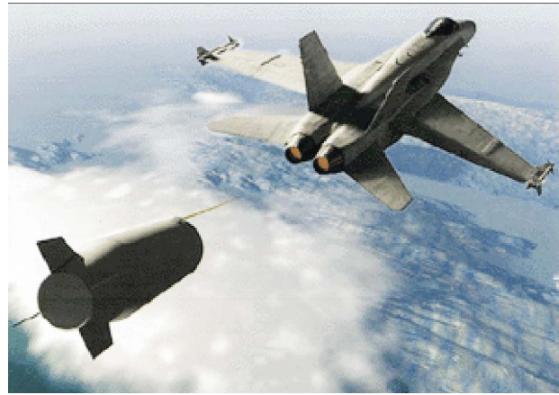
Figure 6. Example of an off-board jammer: an F/A-18 Hornet towing an AN/ALE-50 towed decoy. (Reproduced with permission from the U.S. Navy's Office of Information.)
