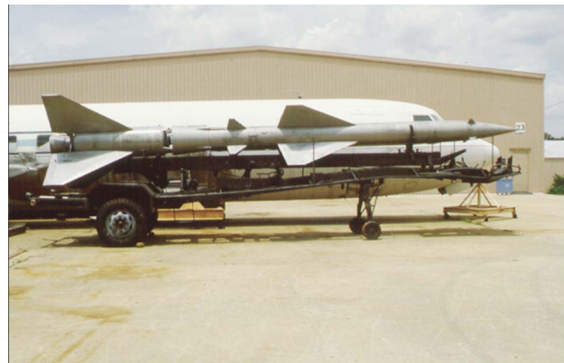
Figure 2. Example of a medium-range SAM system: an Iraqi SA-2. (Reproduced with permission from the National Air and Space Museum.)
