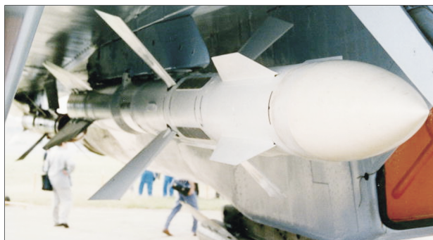
Figure 4. Example of an air-to-air missile: an AA-10 "Alamo" on an ejection launcher under an Su-27 "Flanker" aircraft. (Reproduced with permission from Jane's Information Group.)
