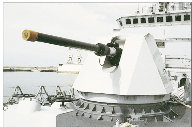
Figure 5. Example of a naval gun system: OTO Melara's 127-mm/54-cal lightweight gun mounted on-board the Italian frigate Bersagliere . (Reproduced with permission from Jane's Information Group.)
