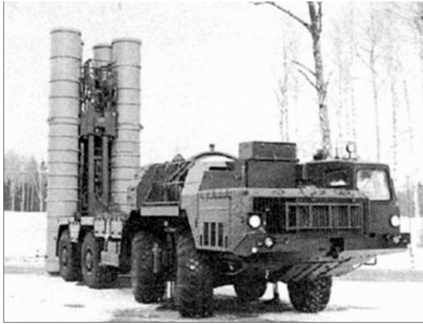
Figure 3. Example of a long-range SAM system: an SA-10 transporter-erector-launcher vehicle with the four missile canisters in the vertical position ready for launch. (Reproduced with permission from the Expeditionary Warfare Training Group, Pacific.)
