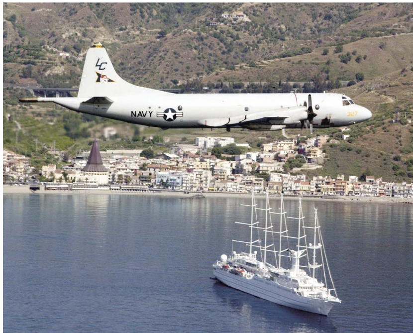
Figure 1. A P-3C Orion aircraft assigned to the “Tigers” of Patrol Squadron Eight (VP-8) flies along the coastline of Taormina, Sicily. The P-3C is a four-engine turboprop anti-submarine and maritime surveillance aircraft. (Photo by Photographer’s Mate Airman Shannon R. Smith.)
