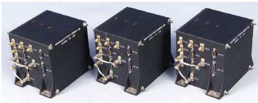
Figure 10. Three NanoSat Cross-Link Transceiver (NCLT) systems as delivered to Goddard Space Flight Center in 2003 that will provide modular, integrated GPS navigation and cross-link communication among a formation of satellites.
