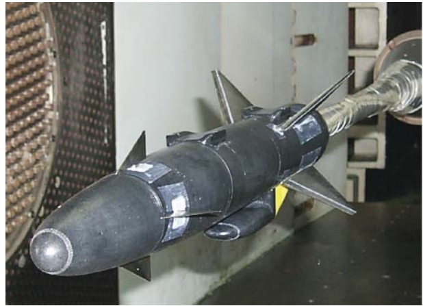
Figure 4. Scale-model missile airframe fabricated using the hybrid rapid prototype process tested up to transonic speeds in a wind tunnel.
