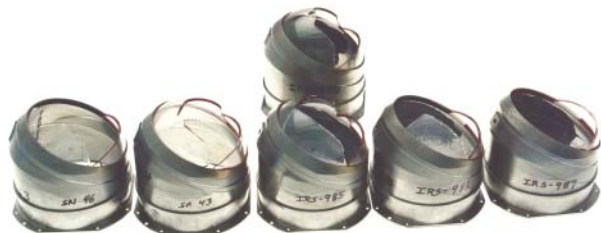
Figure 5. Catastrophic failure of an IR dome results from aero-thermal shock under high-speed conditions simulated in APL wind tunnel testing.
