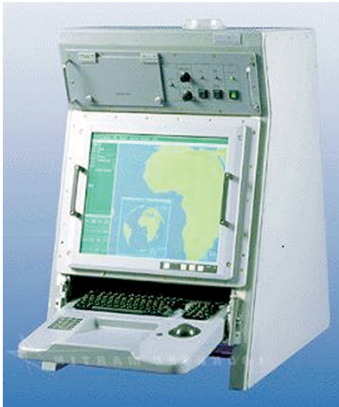
Figure 4. The ACIS airborne Q-70 display console referred to as "bullnose" after its characteristic shape.
