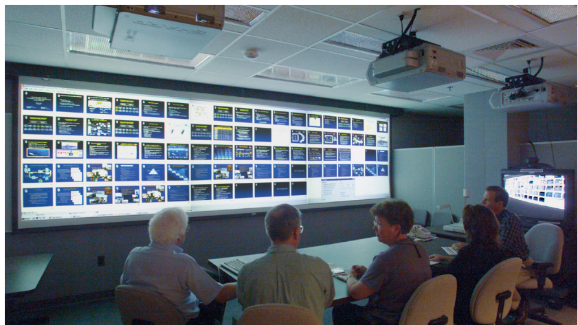
Figure 5. SCDL Electronic War Room space. A 5 \times 17 ft screen driven by a special graphics board supports war room and collaborative engineering. VTC links to outside meeting participants. Presentations are shared using collaborative conferencing software.
