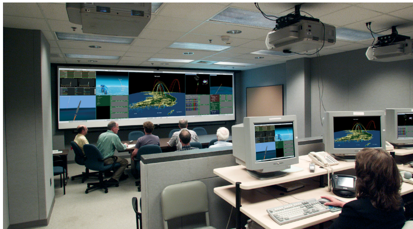
Figure 6. SCDL System Element M&V space. A 5 × 17 ft screen supports three pictures generated by three separate high-fidelity models, and/or multiple views of data generated by a single model. High-end Silicon Graphics computers, Sun workstations, and a 32-PC cluster support a wide variety of engineering-level models and associated visualizations.
