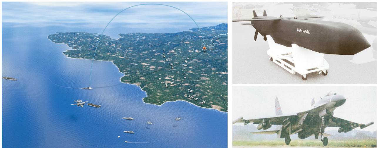
Figure 5. Overland defense of forces ashore (left) against LACMs (top right) and hostile aircraft (lower right) via Extended Range Standard Missile with active seeker technology.
