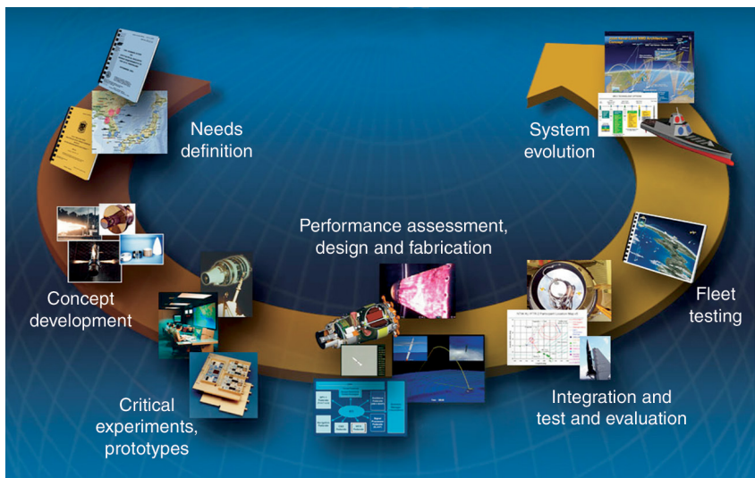
Figure 7. A system development cycle for Sea-Based Midcourse TBMD. The cycle shows systems engineering progression from top-level requirements and concept formulation to Fleet introduction and system evolution.
