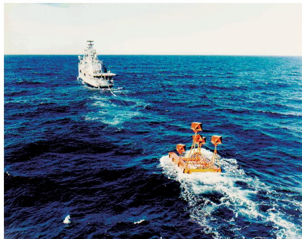
Figure 2. The SDTS tows a target barge during tests to minimize the likelihood that the ship will be hit.
