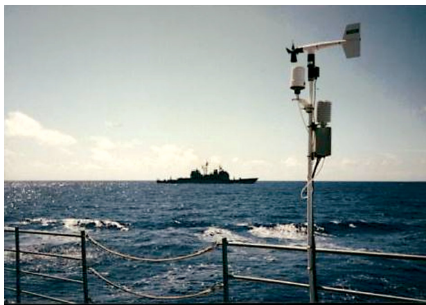
Figure 3. Environmental Assessment System starboard meteorological mast (SEAWASP) on USS Cape St. George during the first Navy shipboard at-sea test, September 1993. USS Ticonderoga is in the background.
