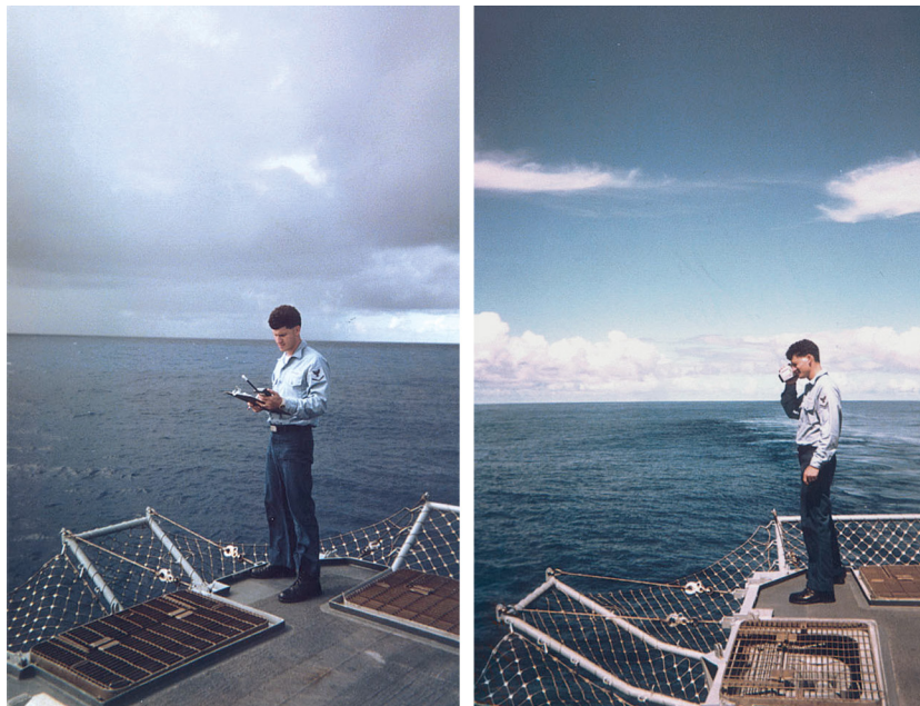
Figure 6. An AN/SPY-1 radar technician uses a thermohygrometer (left) to measure air temperature and humidity and an infrared camera (right) to measure sea surface temperature in support of AN/SPY-1 radar performance assessment via tools and guidance provided in TACMEMO.
