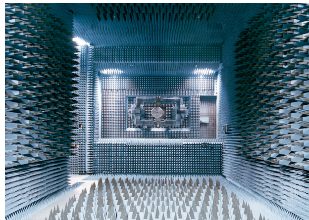
Figure 3. GSEL anechoic chamber in Building 26: the outside north end of the chamber (top) and an inside view looking north toward the test stand where a guidance section would be mounted (bottom).
