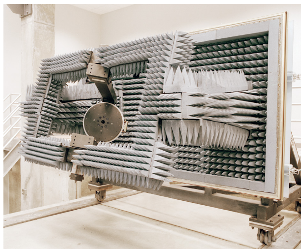
Figure 4. The three-axis test stand, shown pulled back from the anechoic chamber, is used to hold the guidance section under test. The test stand allows movement in the roll, yaw, and pitch rotational axes. The stand is treated with a radar absorber, as is the rest of the chamber, to reduce undesirable reflections.
