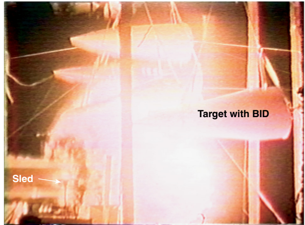
Figure 12. This high-speed photograph shows the target with the BID as the warhead begins to explode.
