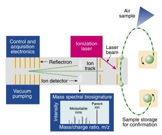
Figure 2. Schematic of a miniature time-of-flight biodetection system developed by APL.
