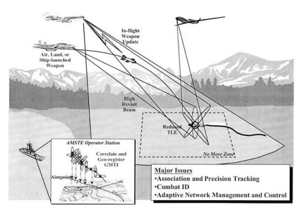
**Figure 3.** The Affordable Moving Surface Target Engagement (AMSTE) System concept (GMTI = ground moving target indicator, TLE = target localization envelope).
