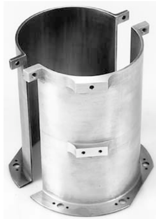
Figure 5. A magnesium battery cell for the TIMED spacecraft that was fabricated using the four-axis machining feature of the Haas V4 milling center.
