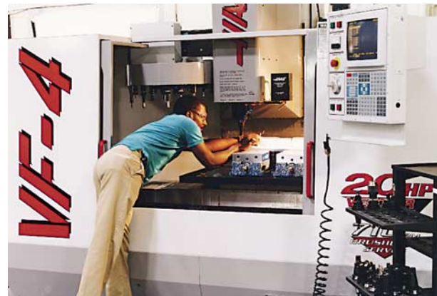
Figure 4. Modern CNC milling machine that includes a powerful controller, an automatic tool changer, and four-axis motion control.
