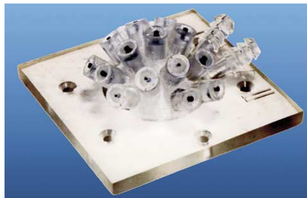
Figure 8. Stereolithography was used to produce this complex vacuum fixture used to hold individual lenses in place for bonding to make a “fly eye” lens assembly.
