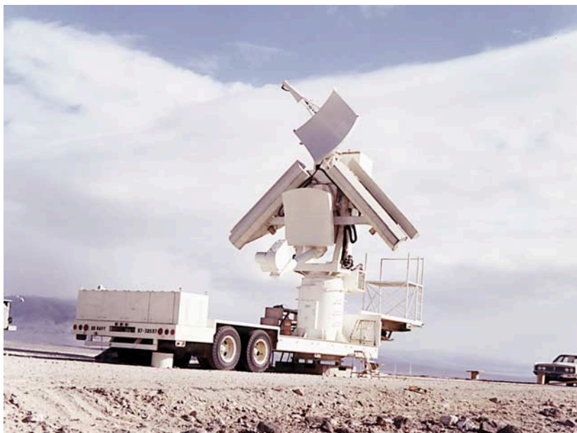
Figure 3. Low Blow simulator antenna system.
