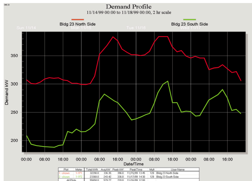
Figure 5. Sample electrical load profile from the networked, solid-state metering system. The profiles show peak demand for power during daily operations in particular buildings. (The profile for Building 23 is shown.)
