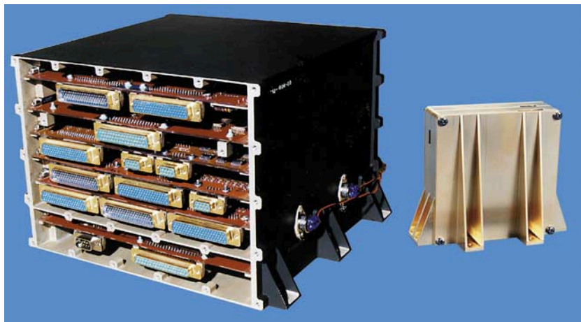
Figure 11. COB implementation of the NEAR Command/Telemetry Processor ( 24 \times 24 \times 17 cm, 5 kg) compared with the palm-sized Command and Data Handling System ( 11 \times 11 \times 5 cm, 0.5 kg).
