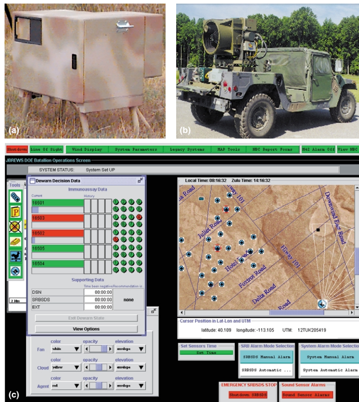
Figure 2. The JBREWS ACTD comprises (a) a point sensor (shown here in field setup), (b) a short-range biological detector mounted on a HUMMWWV, and (c) a SNCP (sensor control screen shown here).
