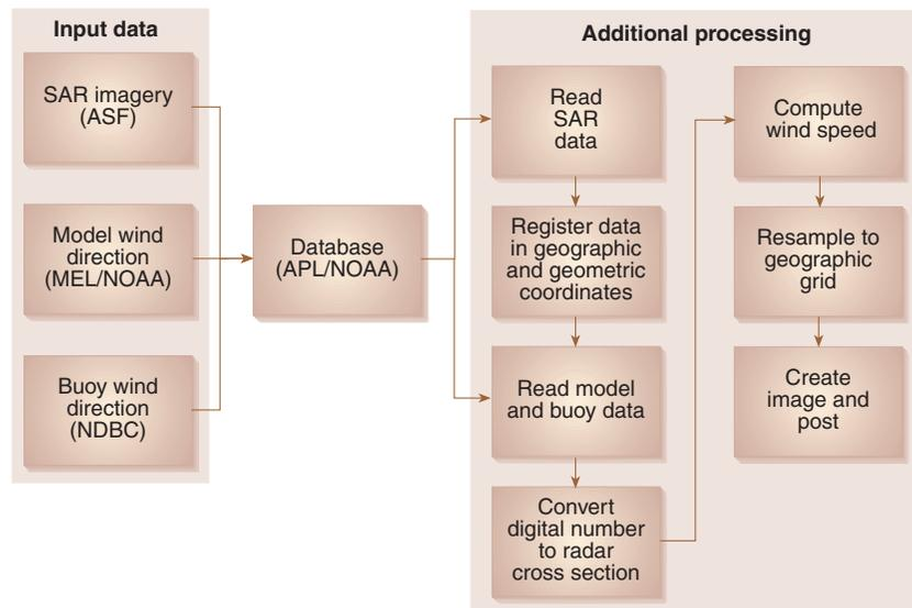
**Figure 2.** Diagram of data flow. (ASF = Alaska SAR Facility; MEL = Master Environmental Library [Navy]; NDBC = NOAA National Data Buoy Center; NOAA = National Oceanic and Atmospheric Administration.)
