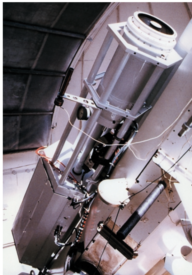
Figure 4. The APL solar vector magnetograph installed at the National Solar Observatory in Sunspot, New Mexico.
