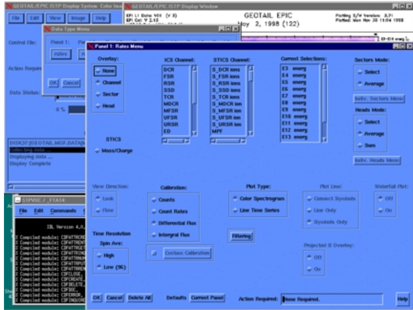
Figure 5. An example of a multiple-window widget interface for a visualization tool. To control display options, the user interacts with a base window and is presented with pop-up windows containing default choices that the user may change.
