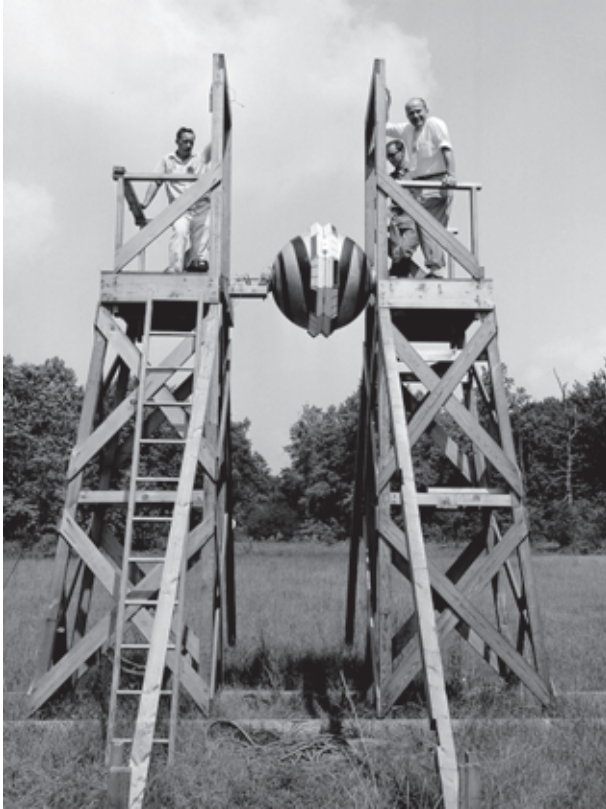
Figure 9. The yo-yo despin mechanism being tested on APL's first satellite in 1959, under our philosophy of "test what you fly, fly what you test." James Smola (extreme right, now retired) is conducting the test.
