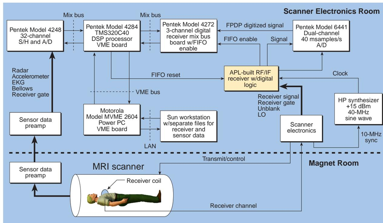
**Figure 1.** Block diagram of the Data Acquisition System. (S/H = sample and hold, A/D = analog-to-digital converter, DSP = Digital Signal Processor, FIFO = first-in/first-out, FPDP = front panel data port, LO = local oscillator, LAN = local area network.)
