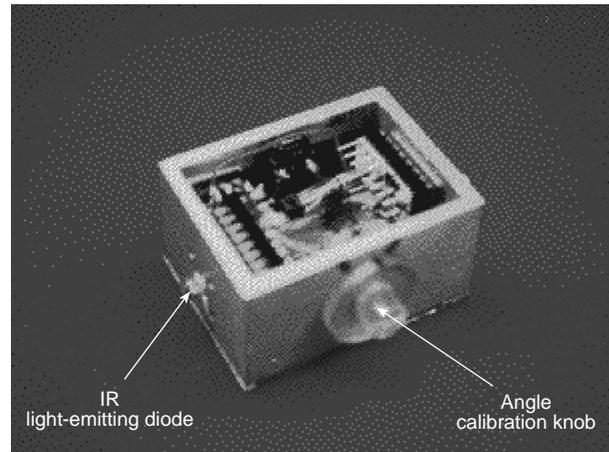
**Figure 6.** Accelerometer sensor and IR transmitter. The enclosure is about 5 cm wide  $\times$  3.8 cm tall  $\times$  3.8 cm deep. A plastic on/off switch is mounted on the back of the enclosure.
