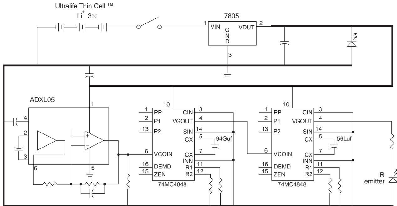
Figure 7. Circuit schematic of the accelerometer and IR transmitter. The ADXL05 was repackaged by APL into a nonmagnetic die.
