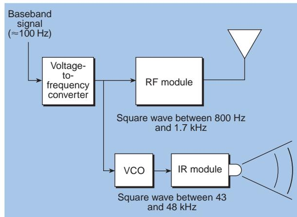
Figure 8. Wireless modulation techniques.
