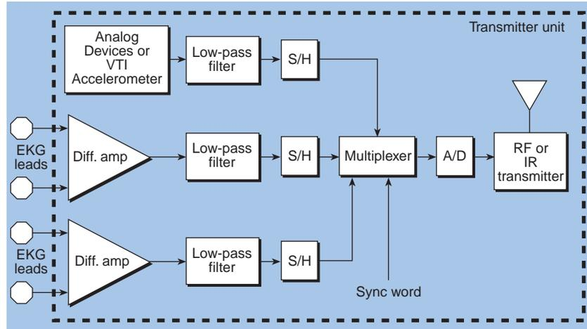
Figure 17. Block diagram of a modular, wireless accelerometer/multiple EKG.
