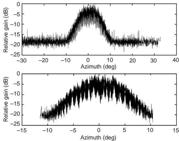
**Figure 5.** Radar azimuth data (operating frequency = 35.4848 GHz with 0° cutting angle).
