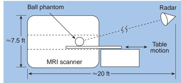
Figure 10. Sketch of the moving table experiment.
