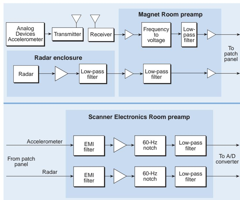
Figure 3. Block diagram of preamps used for radar and accelerometer.
