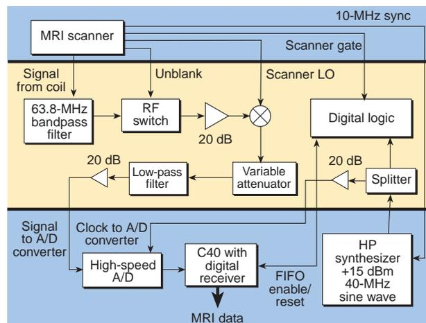
**Figure 2.** Expanded view of the APL-built RF/IF receiver with digital logic shown in Fig. 1.
