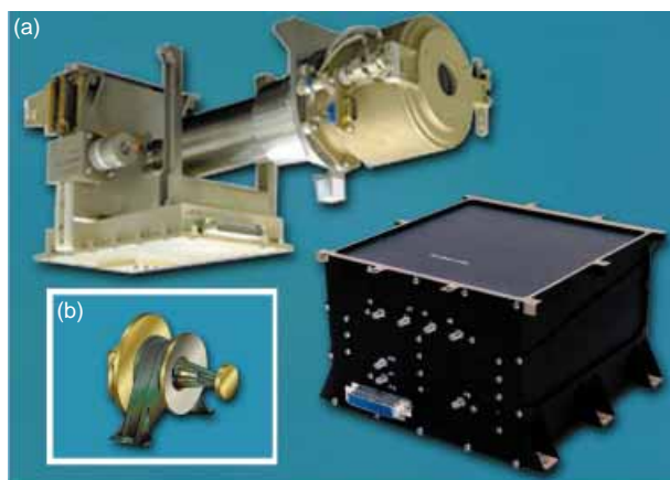
Figure 8. The miniaturized scientific imager. (a) Original design: Total weight = 17.5 lb (sensor = 8.5 lb, digital processor unit = 8.2 lb, harness = 0.8 lb). (b) COB design: Total weight of sensor and control electronics = <1.1 lb.
