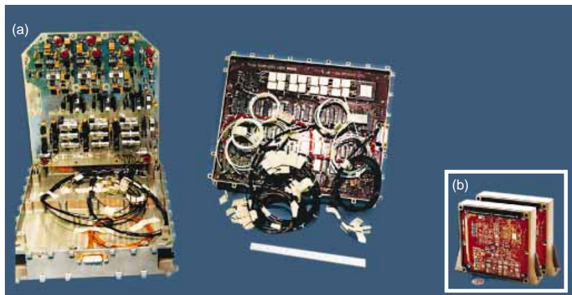
Figure 1. The Freja magnetometer signal processor. (a) Original design: Size = 9.8 \times 7.9 \times 3.54 in.; weight = 6.7 lb. (b) COB design: Size = 4.5 \times 4.5 \times 2 in.; weight = 1 lb.
