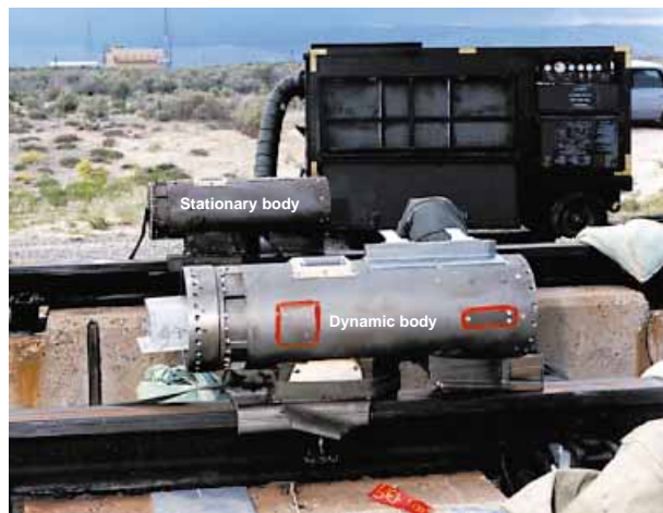
Figure 2. Instrumented bodies during checkout. The dynamic body has S-band and GPS antennas mounted on top; the stationary body has only a GPS antenna. Both bodies have GPS signal translators mounted inside, and the dynamic body also includes internal telemetry functions. Telemetry and translator signals are communicated through the two S-band antennas on the dynamic body. An RF cable carries S-band signals from the stationary body to a track-side block house. The air conditioning unit in the background (used during checkout) was removed before the sled test.
