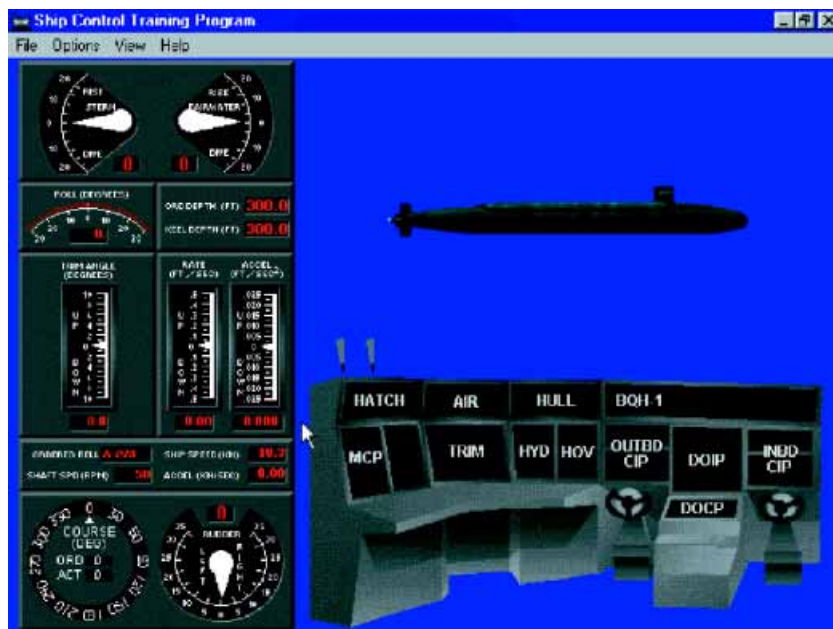
Figure 4. Main SCTP drill-and-practice interface screen providing a summary of the submarine's ship control status and access to ship control console panels. (By clicking on the abbreviated icons on the mock-up of the ship control console, the panels are brought to the foreground.)
