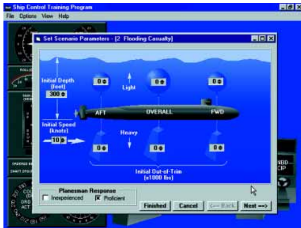
Figure 6. An example of the parameter initialization dialog box providing capability to vary initial conditions and events of an SCTP exercise.
