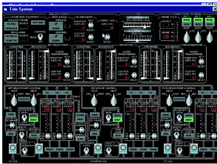
Figure 5. An example of the SCTP replica of a ship's trim system panel on which all indications and switches are active and can be controlled via mouse clicks.
