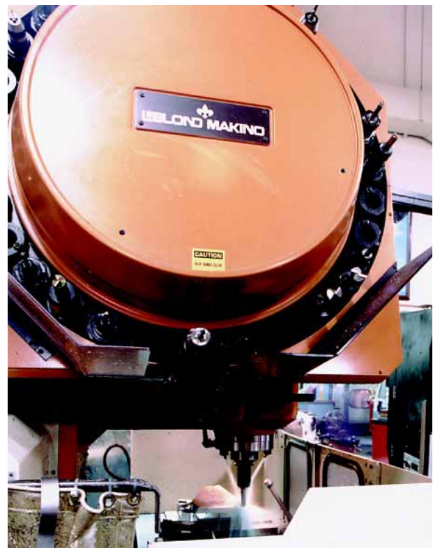
Figure 7. Unattended numerically controlled machining. Note that the tool currently in use has been selected from the tool turret.
