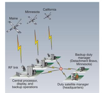
Figure 8. The duty satellite manager at headquarters normally controls all operations. A duty manager at the backup site assumes controls if headquarters is disabled.
