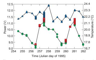
Figure 14. Oscar voltage/temperature curves depicting effects of daily switching of boost array between main bus and automatic temperature control circuits. This switching prevented high battery temperatures while maintaining sufficient charge. (Red data points = battery voltage boost on, green = boost off, blue = average battery temperature.)
