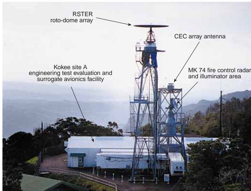
Figure 3. Kokee Park “surrogate” aircraft site A, at a 3800-ft elevation. In addition to providing the surrogate forward pass aircraft functions, test data evaluation of the site elements and the CEC was conducted here. The system elements are described in the text.
