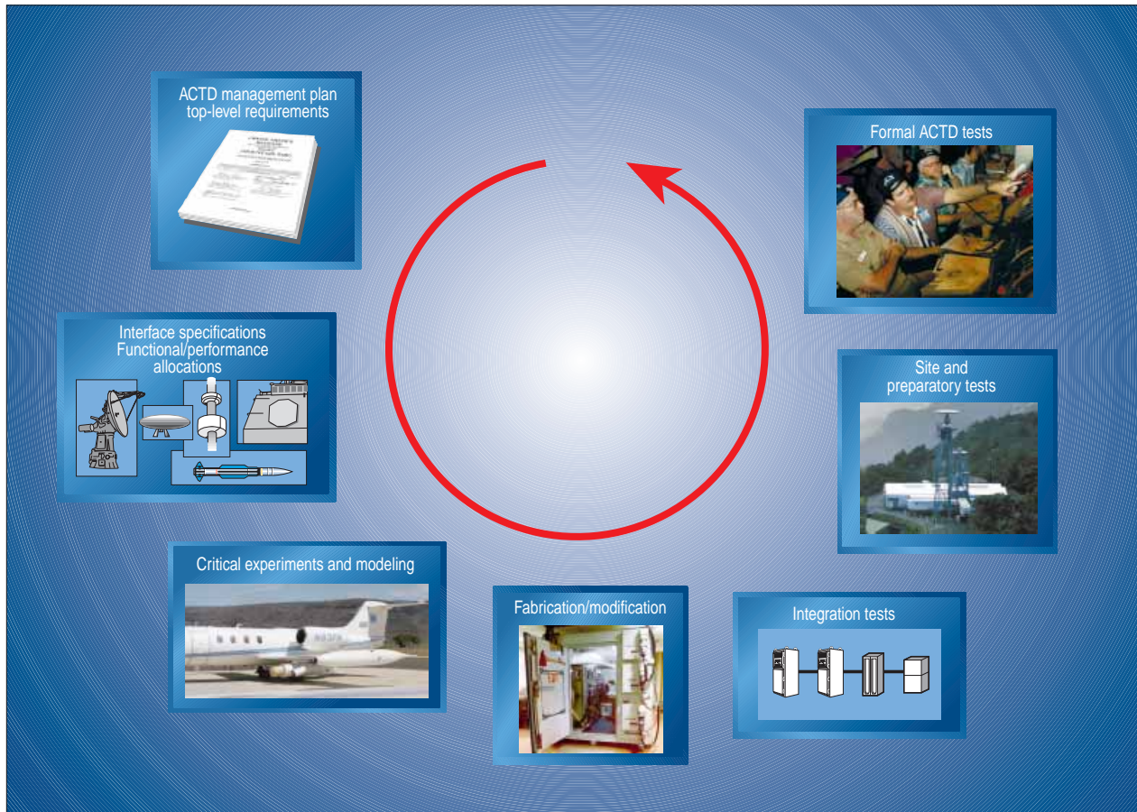
Figure 4. The systems engineering process as applied to the Mountain Top ACTD, beginning with the concept and requirements definition, proceeding through requirements allocation to the elemental level, and finally to testing from the smallest elements up to the fully networked composite system. APL provided leadership in modeling, requirements definition and allocation, interface specifications, critical experiments, site risk reduction scenarios, site subsystem checkout and verification, and test conduct. Shown in the formal ACTD test inset, from right to left, are APL’s Test Conductor, Art Jeyes, sitting beside the CEC and Mountain Top Program Manager, Michael O’Driscoll, and RADM Timothy Hood, the Program Executive Officer for Theater Air Defense.
