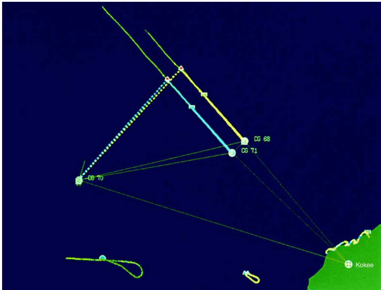
Figure 11. CEC snapshot of dual cooperative engagement events by two firing ships—the USS Anzio (CG 68) and Cape St. George (CG 71)—engaging drones using the USS Lake Erie (CG 70) SPY-1B remote data. The triangles are the drone targets. The CEC-equipped units are circles. The upper-half squares near the drones are SMs in flight. The dotted lines between CG 70 and the targets indicate that CG 70 is the source of fire control data. The solid lines between CG 68 and 71 and the drones indicate the target/ship engagement pairings. The thin solid lines indicate direct CEC connectivity among CEC units.
