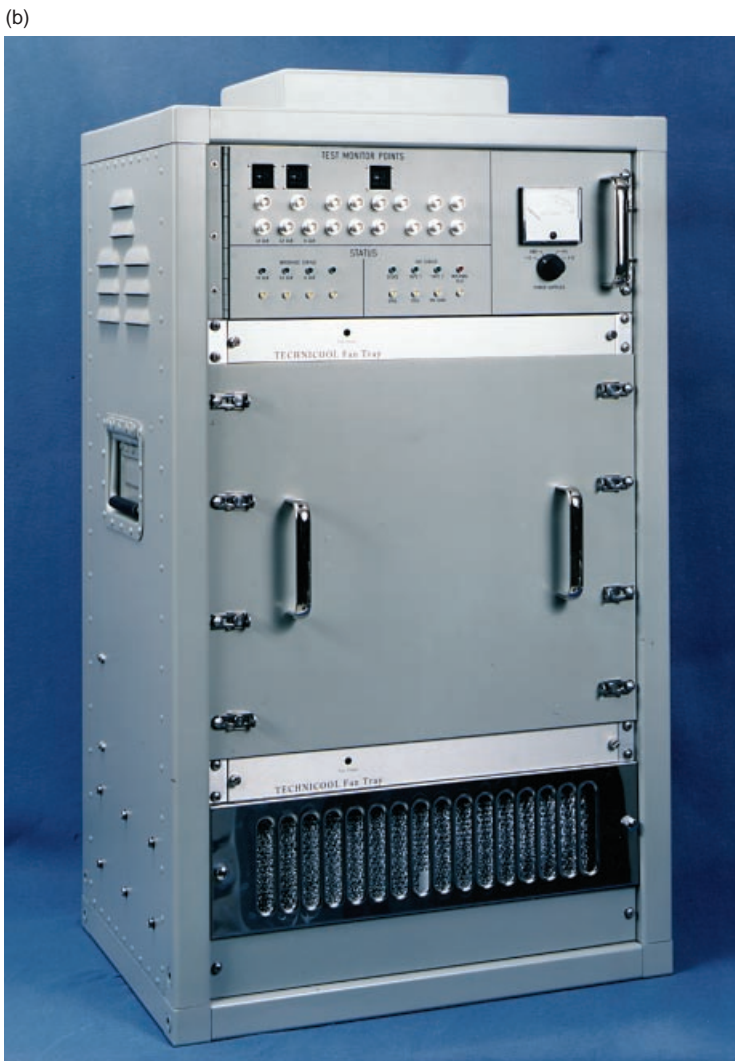
Figure 2. Upgraded Phalanx CDC installation. (a) Conceptual block diagram. The analog buffered IF and LO signals are no longer used; the digital I/Q data signals are sent directly from the search radar to the CDC processor. The interface buffer unit is used solely to send search antenna position information to the CDC processor. The radar interface unit is no longer used. (b) Photograph of the upgraded CDC processor. Its enclosure is the same size as that of the first collector, but the electronics are more sophisticated. The front panel contains test points and status lights only. Control is provided by a control terminal.
