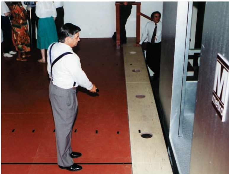
Figure 6. Joe Abita at IRIIS Junction, APL: (a) using the platform edge detector and (b) adjusting the emitter assembly for the open-door detector.
