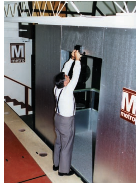
Figure 6. Joe Abita at IRIIS Junction, APL: (a) using the platform edge detector and (b) adjusting the emitter assembly for the open-door detector.
