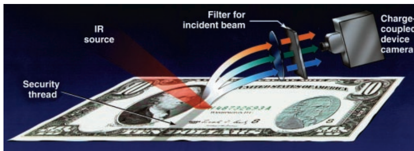
Figure 4. Probing currency using phosphor embedded in security thread.
