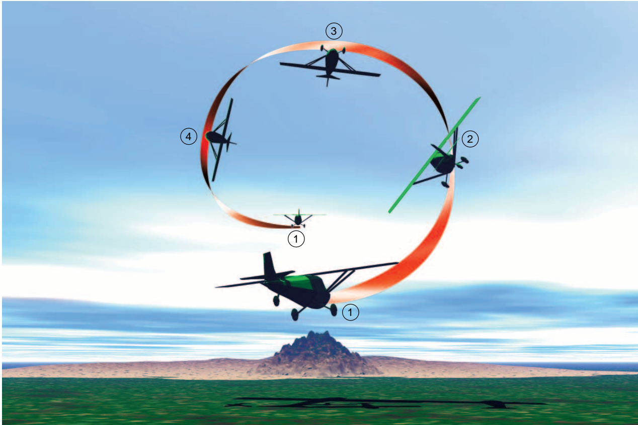
Figure 10. The barrel roll viewed from behind the aircraft. Positions correspond to those shown in Fig. 9.
