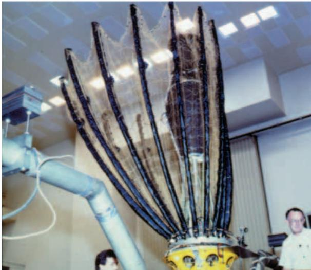
**Figure 6.** Galileo's main antenna. (a) The Galileo spacecraft in an environmental chamber with its high-gain antenna unfurled. (b) The most likely configuration of the high-gain antenna following its unsuccessful deployment in April 1991. The analysis of data from the spacecraft and laboratory tests using a spare antenna showed that three ribs on the main antenna are stuck, keeping the antenna from deploying.
