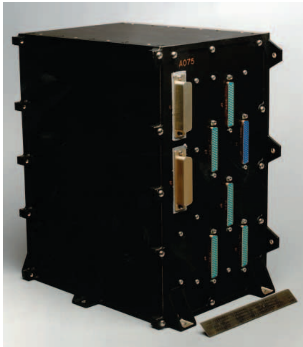
Figure 2. View of the command processor showing the connector panel.
