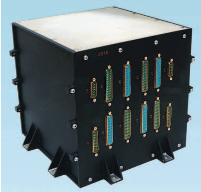
Figure 6. Front view of power switching unit 1, showing the connector panel.
