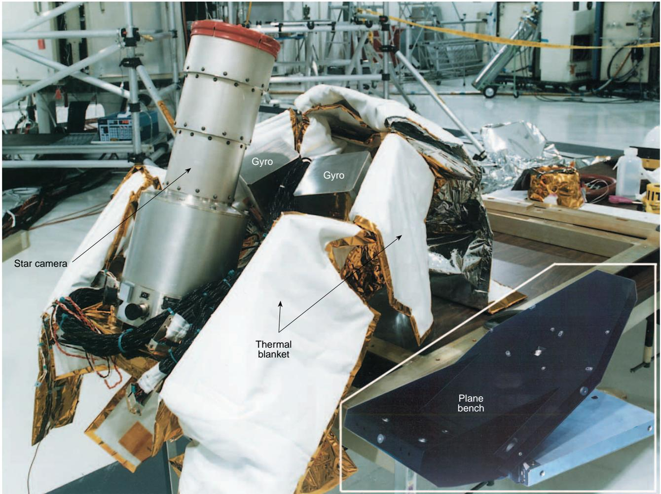
**Figure 13.** MSX optical bench (structure shown in lower right).
