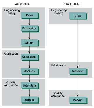
Figure 9. Comparison of old and new heat-sink development processes at APL.
