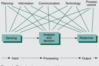
Figure 1. Three-function systems model.
