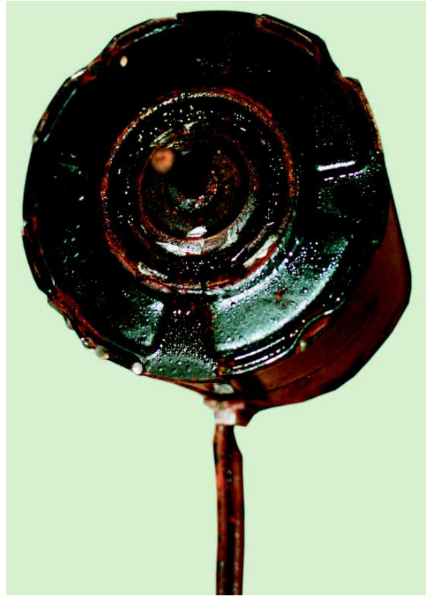
Figure 15. This inexpensive motor with badly corroded exterior remains operable and safe after 2258 h under water.
