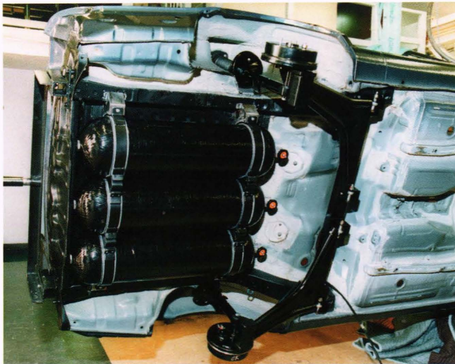
Figure 4. Form/fit check of the trailing-arm rear-suspension and underbody storage assemblies on the chassis mock-up.
