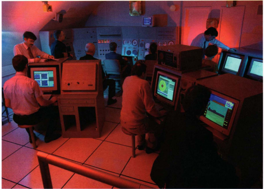
Figure 2. The Submarine Combat Information Laboratory (SCIL). This facility, a mockup of a submarine control room, creates a sense of being aboard ship. Control console displays enable operators to interact in the SCIL's virtual world.
