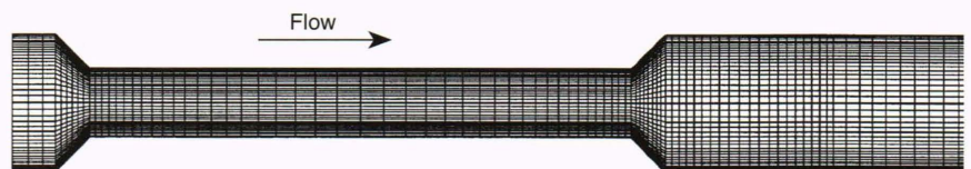
Figure 4. Finite element grid near a constriction.
