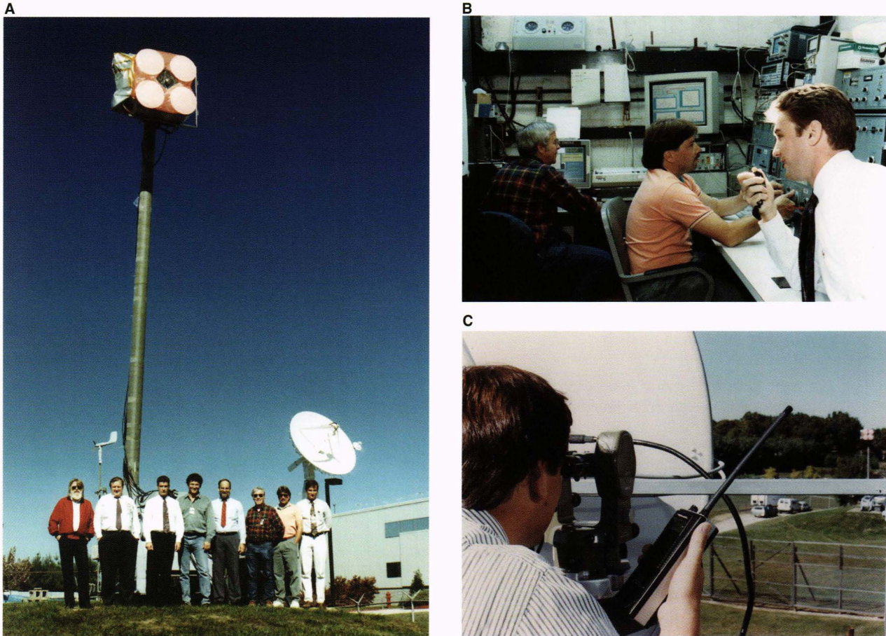
Figure 14. Flight hardware boresight calibration of the Beacon Receiver at the Space Department antenna range. A. Beacon Receiver antenna assembly mounted on the antenna range positioner tower. Assembled test and analysis team includes (L-R) R. K. Stilwell, M. L. Edwards, T. R. McKnight, C. R. Valverde, J. R. Jensen, R. F. Platte, J. T. Will, and C. C. DeBoy. B. T. R. McKnight conducts Beacon Receiver tests while R. F. Platte controls the Beacon Receiver via its ground support equipment and J. T. Will operates the antenna positioner. C. C. C. DeBoy uses a theodolite to boresight the Beacon Receiver at the desired angle offset from the simulated target beacon.
