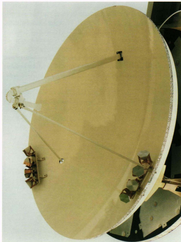
Figure 7. The Spinsat Radar Altimeter (SALT) flight antenna. The antenna consists of a 36-in.-dia. parabolic reflector with a compound rectangular horn feed. A laser reflector array is installed on the reflector to save space; the resulting aperture blockage decreases antenna gain only slightly.
