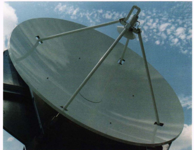
Figure 4. The radar altimeter flight antenna for the Ocean Topography Experiment (TOPEX)/Poseidon satellite. The antenna consists of a 1.5-m-dia. reflector with a dual-frequency, three-port feed. Dual orthogonally polarized signals are launched via an orthomode transducer (see Fig. 5).
