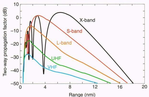
**Figure 9.** The low-elevation two-way propagation factor is shown for several frequencies at a radar antenna height of 100 ft for a sea-skimming cruise missile at a 12-ft altitude. The X-band advantage over S- or L-band at a detection range of 10 nmi is as great as 16 or 27 dB, respectively.
