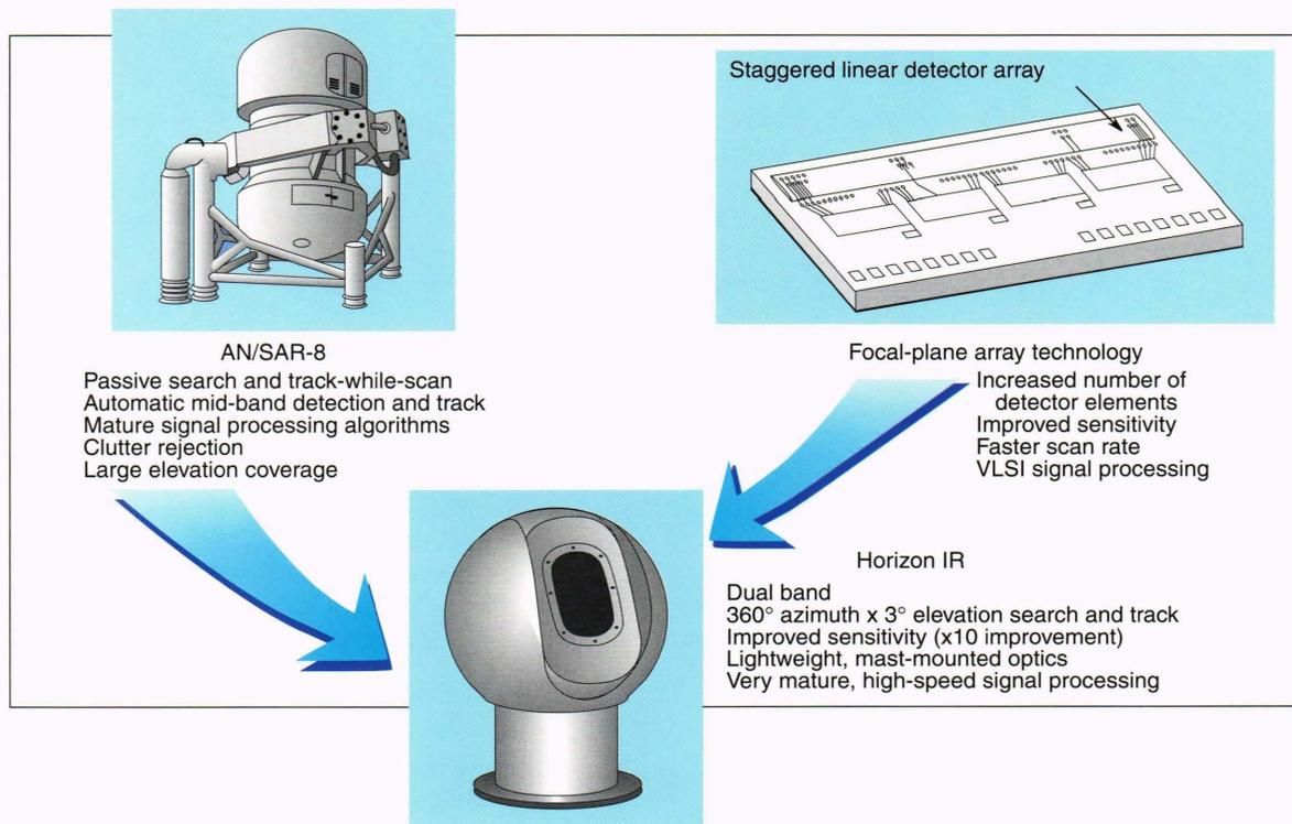
**Figure 11.** Engagement battlespace lost owing to the high-speed, low-altitude, and small radar-cross-section supersonic cruise missile can be regained through multispectral data fusion and radar cueing using focal-plane-array IR sensor technology with improved sensitivity and a faster scan rate. Lightweight optics permit high mast mounting, which further extends the horizon and detection range against the high-speed (thus "hot" IR signature) threat. VLSI = very large scale integrated circuit.
