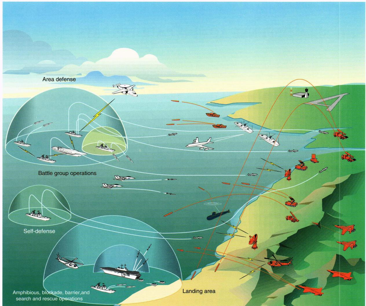
**Figure 1.** Air defense in the littoral environment includes defense against cruise missiles, ballistic missiles, and aircraft in the diverse, dense-air-traffic, and cluttered near-land setting. A robust integral self-defense capability must provide a final layer of defense in joint expeditionary and traditional battle group operations as well as an autonomous capability for ships operating alone.
