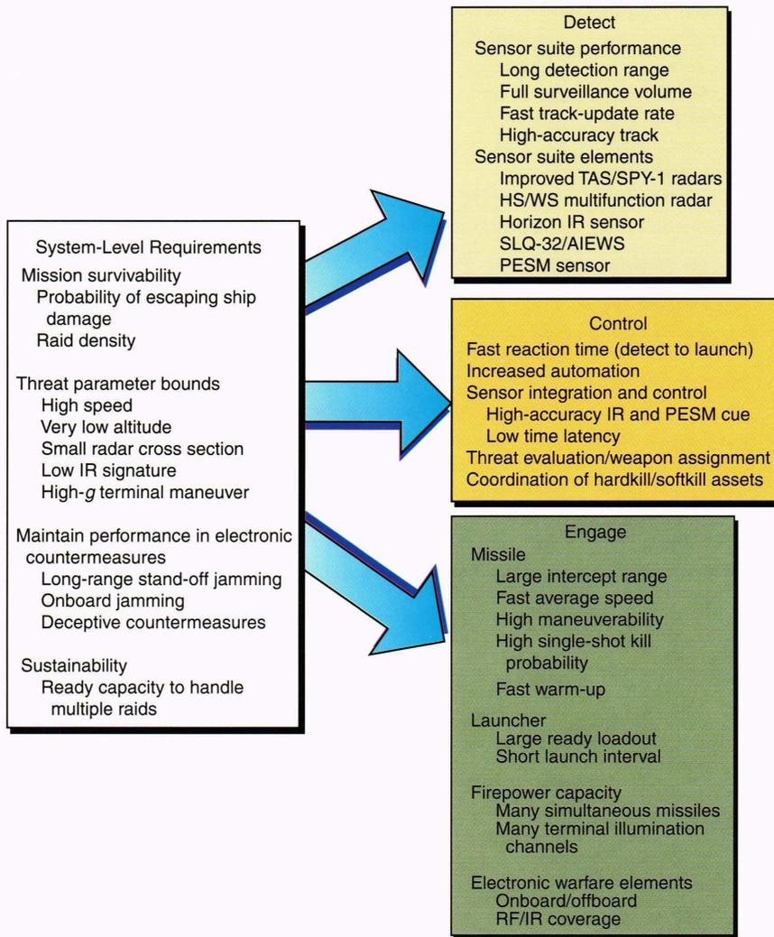
**Figure 5.** The overall combat system mission-survivability requirements can be allocated to the major elements (detect, control, engage) of the weapon system. The individual element requirements and threat parameter bounds determine the necessary technology and the extent of the modifications required. TAS = Target Acquisition System, HS/WS = Horizon Search/Weapon Support, AIEWS = Advanced Integrated Electronic Warfare System, PESH = Precision Electronic Support Measures.
