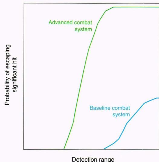
**Figure 4.** The projected combat system performance against multiple advanced low-altitude, supersonic, maneuvering cruise missiles depends on the detection range as well as the system reaction time, defensive missile launch rate, flight time to intercept, endgame effectiveness, and number of available illumination channels. Adequate performance can be achieved with detection, command and control, defensive missile, and electronic warfare upgrades associated with the advanced combat system.
