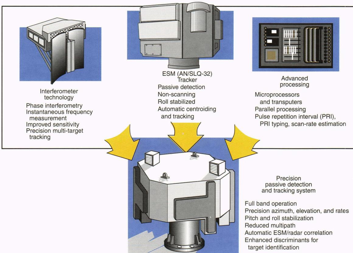
**Figure 12.** As with the horizon IR sensor (Fig. 11), precision electronic support measures data can extend detection ranges and enhance defense against cruise missiles through data fusion and cueing. Interferometer technology enables improved sensitivity; precision azimuth, elevation, and rate tracking; and enhanced discriminants for target identification. ESM = electronic support measures.
