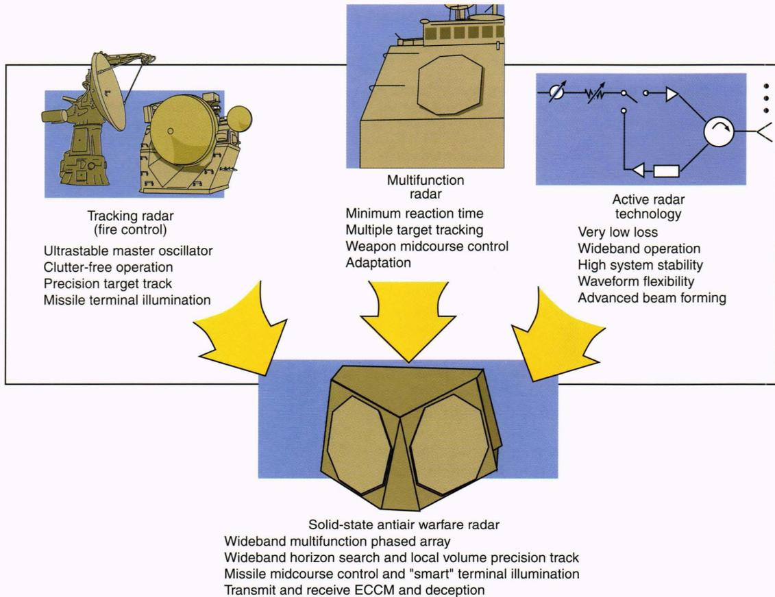
**Figure 10.** The Horizon Search/Weapon Support multifunction radar is a mix of old and new technologies. The application of solid-state, active-element radar technology significantly enhances performance in terms of low loss, high stability, wideband operation, waveform flexibility, and electronic countermeasures resistance. ECCM = electronic counter countermeasures.
