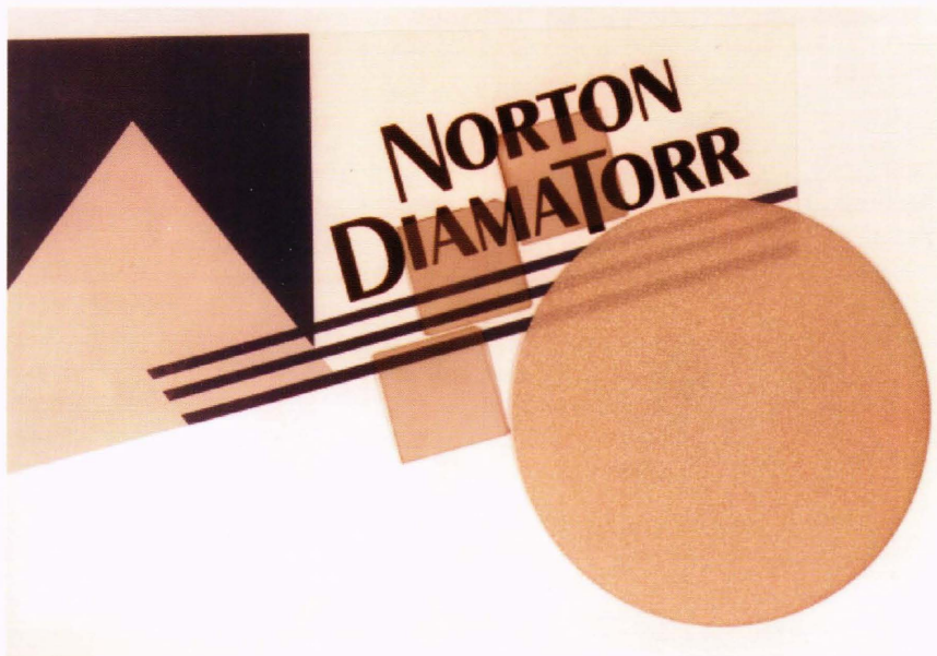
Figure 1. Polycrystalline diamond windows made by Norton (DiamaTorr process). The square windows are 1 in. on a side and are polished; the 4-in. circular wafer is unpolished. All samples are about 0.5-mm thick. The slight brown coloring is due to scatter. (Photograph courtesy of the Norton Diamond Film Company.)
