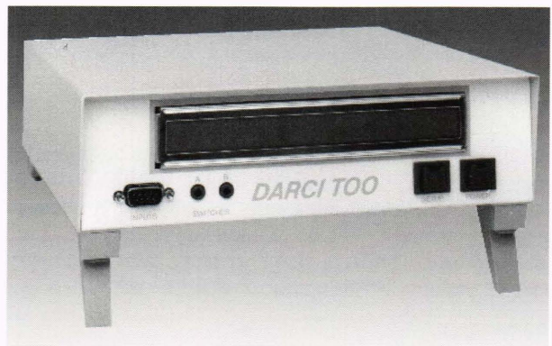
Figure 1. DARCI TOO: an alternative computer input device for disabled people.
