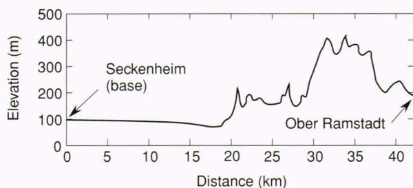
**Figure 13.** Terrain profile for a high-frequency ground wave path in Germany over which digital weather data were passed at a baud rate of 2400.
