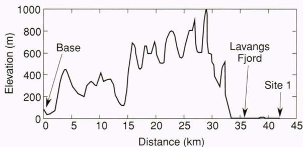
**Figure 8.** Terrain profile for the high-frequency ground wave path from base to site 1 near Santorg, Norway.
