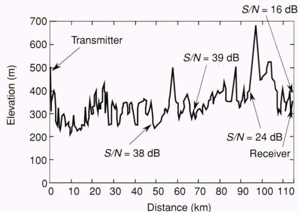
**Figure 7.** Terrain profile for path 4 across the mountains west of the Rhine shown in Figure 5. S/N = signal-plus-noise to noise ratio.
