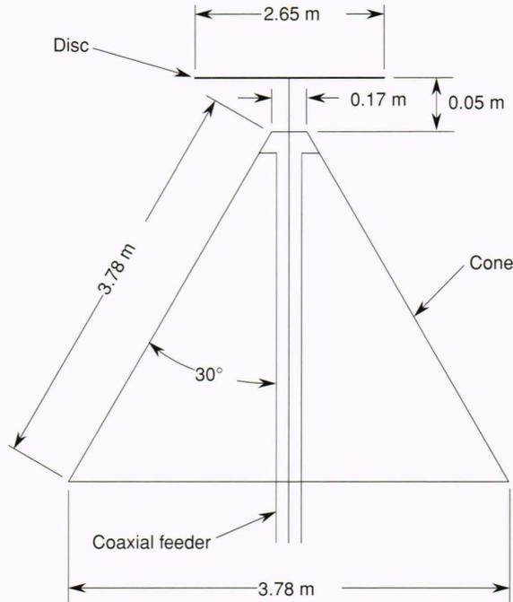
**Figure 3.** Dimensions for a discone antenna with a cutoff frequency of 19 MHz.
