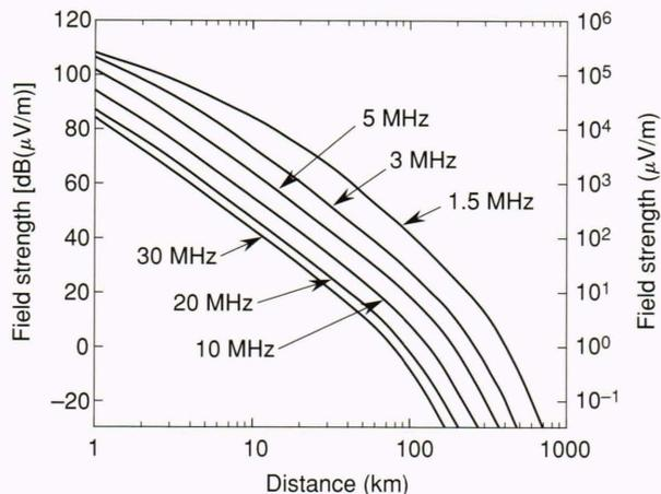
**Figure 2.** Ground wave propagation curves for wet ground (conductivity =  $10^{-2}$  s/m, dielectric constant = 30). Provided by the International Radio Consultative Committee.
