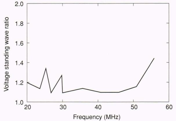
**Figure 4.** Voltage standing wave ratio versus frequency for a discone antenna with a cutoff frequency of 19 MHz.
