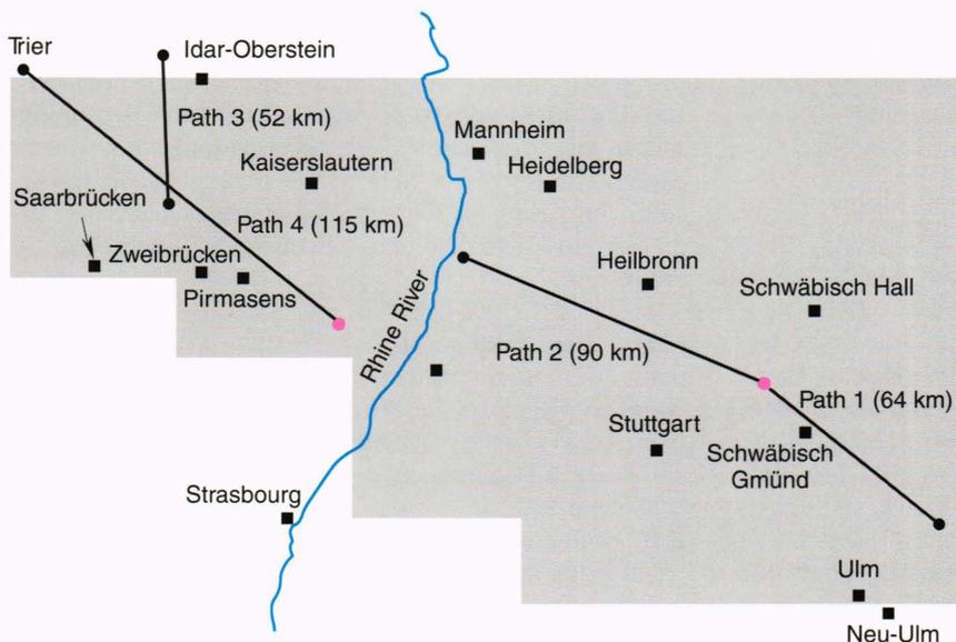
**Figure 5.** Map showing region of four high-frequency ground wave test paths listed in Table 1. The transmitting antenna was placed at the sites designated in red. The paths surveyed are represented by the black lines.
