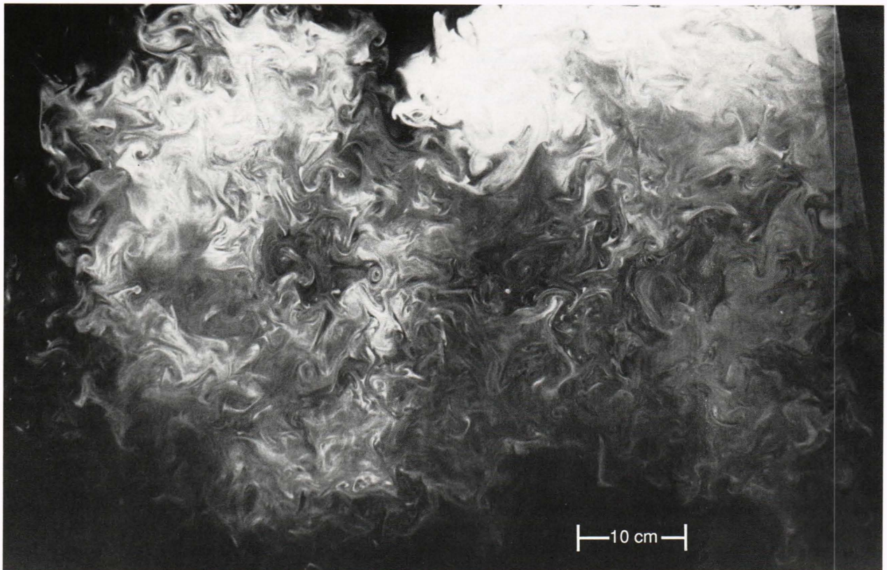
Figure 4. Turbulence-induced microstructure produced in the Hydrodynamics Research Laboratory's recirculating flow channel. Fluorescein dye injected from a grid upstream and illuminated by a laser sheet across the 88 \text{ cm} \times 56 \text{ cm} cross section of the channel visually demonstrates the wide range of scales present in turbulence-induced microstructure.
