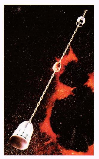
**Figure 7.** The first drag-free satellite, Triad. The central unit contains the DISCOS (Disturbance Compensation Device). The Earthpointing portion (bottom) carries nested quadrifilar helix antennas. The top unit contains the nuclear power supply, the last of six flown by APL.
